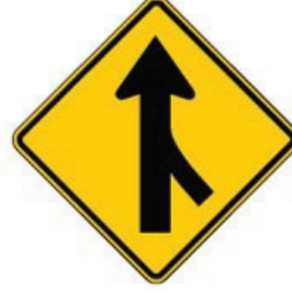
ACCESS LANE/RAMP MERGES INTO ROAD- WAY (from right).
