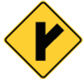
SIDE ROAD enters from angle ahead.
