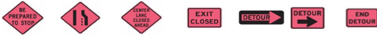
Be Prepared to Stop Lane Ends Center Lane Closed Ahead Exit Closed Detour Detour End Detour
